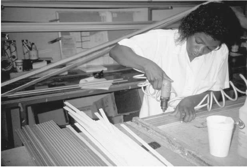
Figure 16-3. In jobs like this, reducing the load on the wrist, elbow, and shoulder can be accomplished by one or more of the following three methods: changing the tool, reorienting it (from vertical to horizontal, or vice versa), and changing the height of the work station—either elevating the worker or lowering the piece being worked on. (Courtesy of Washington Industrial Safety and Health Act Services Demonstration Project.)
