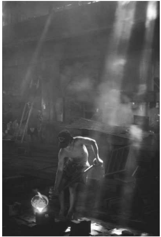
Figure 11-4. A barefoot worker pours molten iron into molds in a foundry in the Philippines as sunlight penetrates the emission-laden atmosphere containing carbon monoxide, crystalline silica, hydrocarbons, and carbon particles. The foundry was studied as part of an International Labor Organization–sponsored industrial hygiene course for government labor inspectors. (Photograph by Aaron Sussell.)
