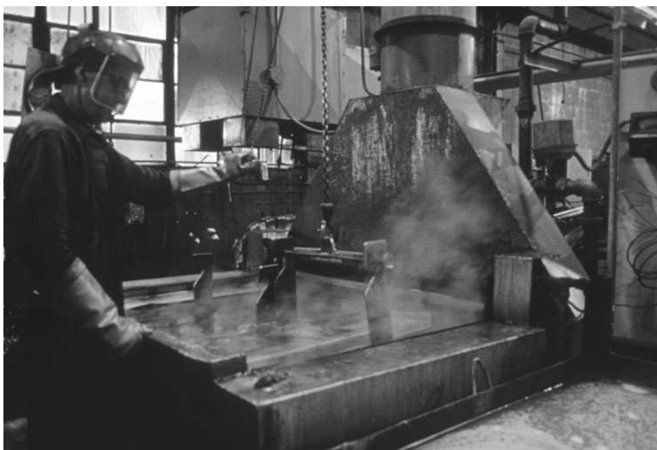
Figure 26-5. Electroplating workers are protected by local slot exhaust ventilation. (Source: W. A. Burgess, Harvard School of Public Health, Boston, Massachusetts.)
