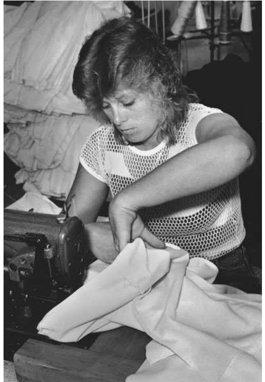
Figure 27-8. Garment workers must repetitively use awkward wrist and shoulder postures when operating sewing machines. (Photograph by Earl Dotter.)
